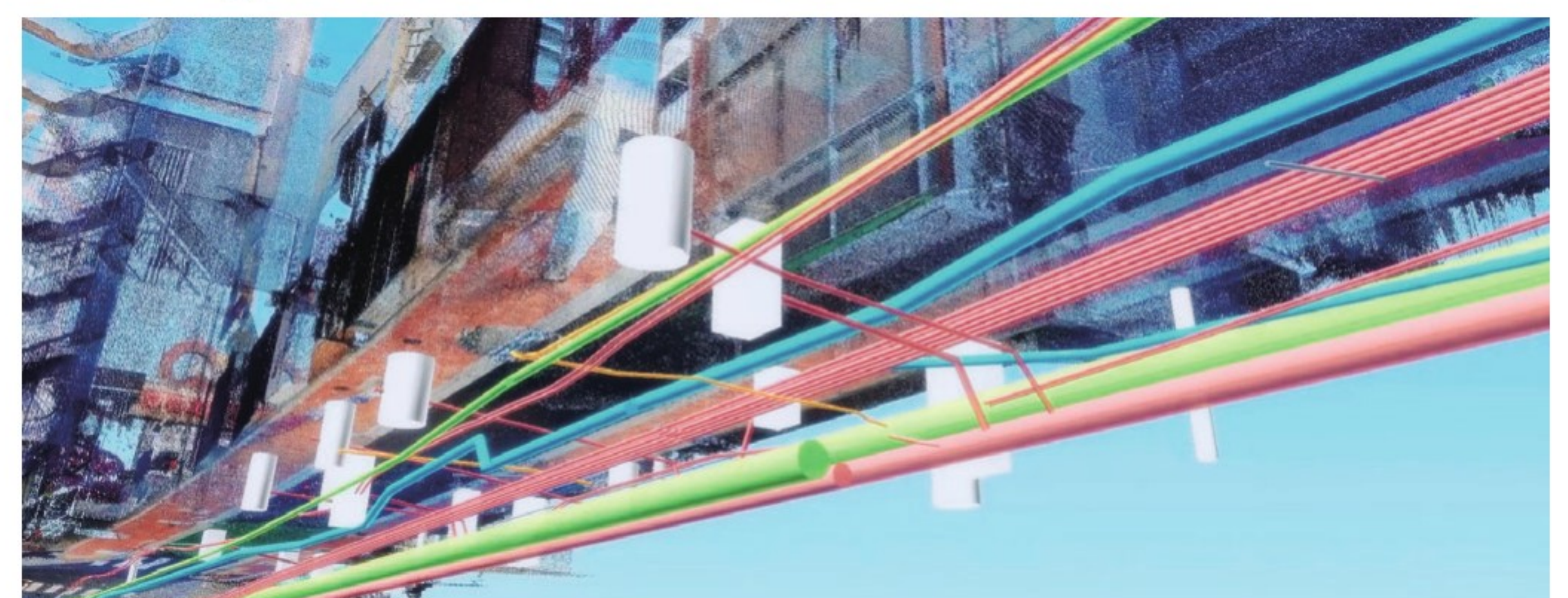
Hybrid 3D map (GPR result with Point-cloud data)
